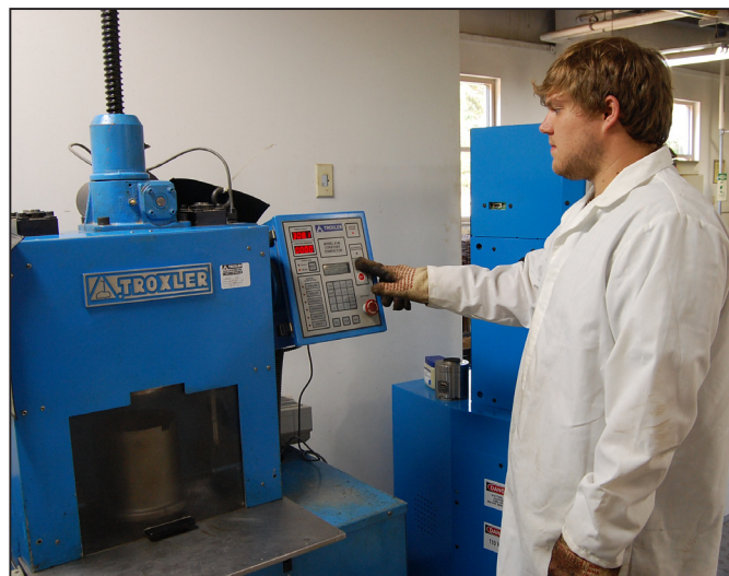
Figure 1 An NCAT lab technician prepares to compact a sample using a Superpave gyratory compactor (SGC).
