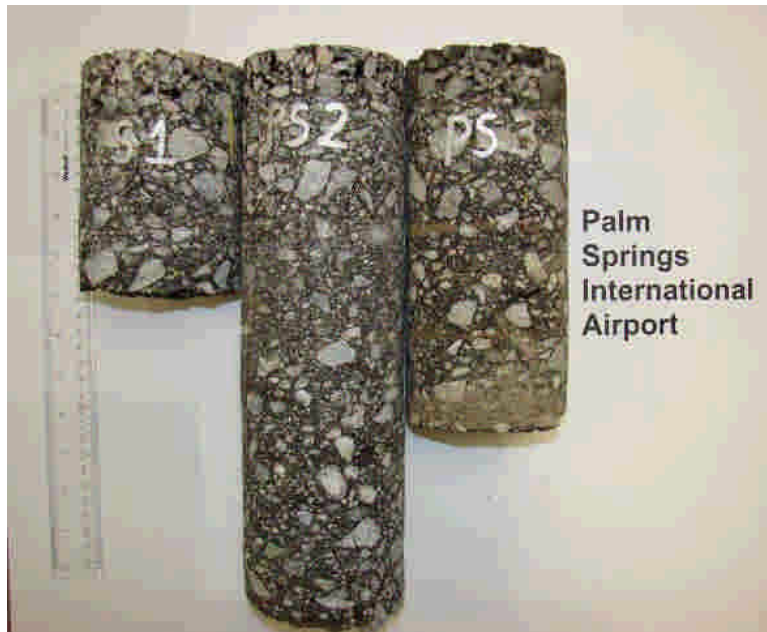
Figure 33: Cores Taken from Palm Springs Runway 13R/31L
