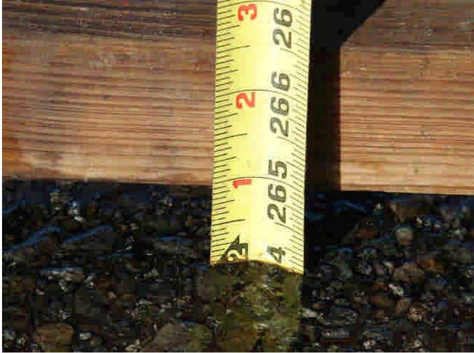
Figure 19: Rut Depth of One Inch
