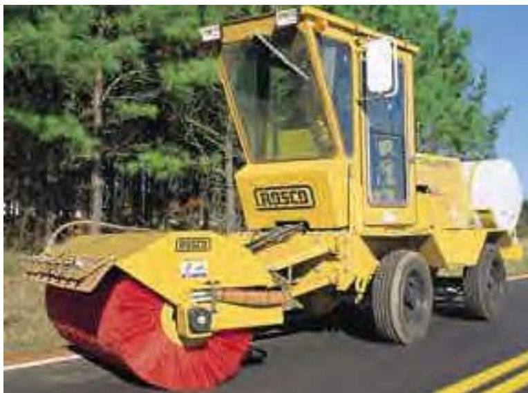
Figure 4.42 Kick Broom Used for Chip Seals
