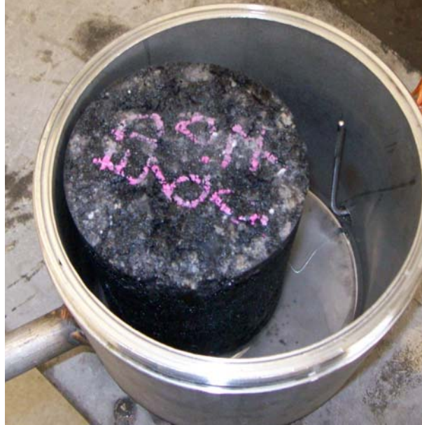
Figure 60. Compacted HMA made with ED RCA after Testing in Deicer Solution at 60°C
