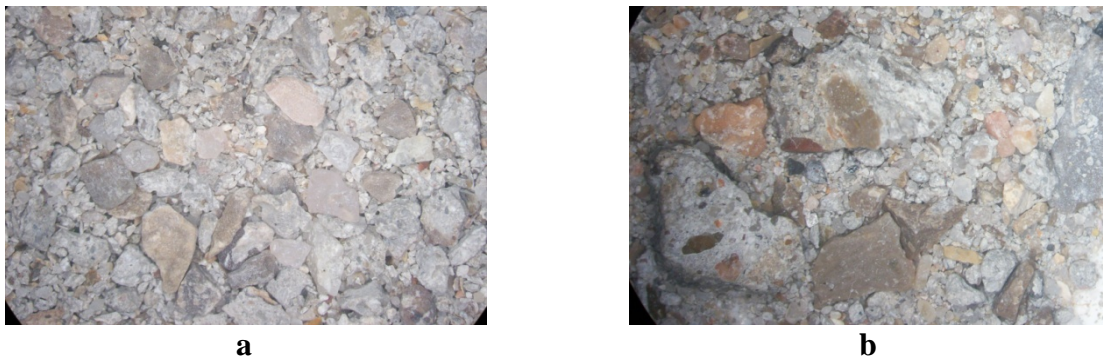
Figure 84. Stereomicroscope Images of Fine HL RCA Particles (a) Before and (b) After Micro-Deval Testing
