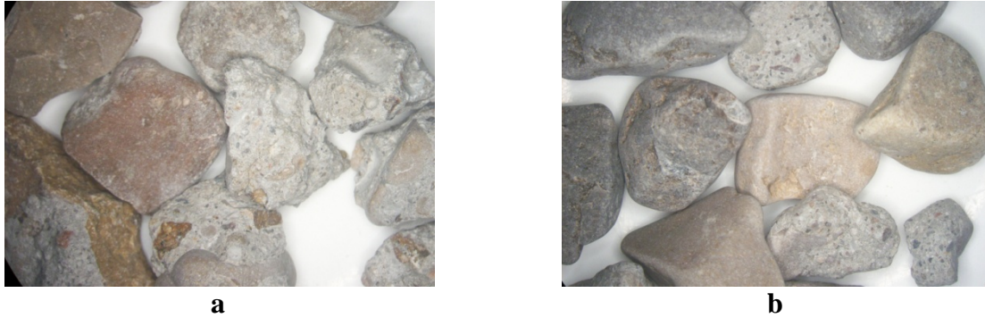
Figure 83. Stereomicroscope Images of Coarse HL RCA Particles (a) Before and (b) After Micro-Deval Testing
