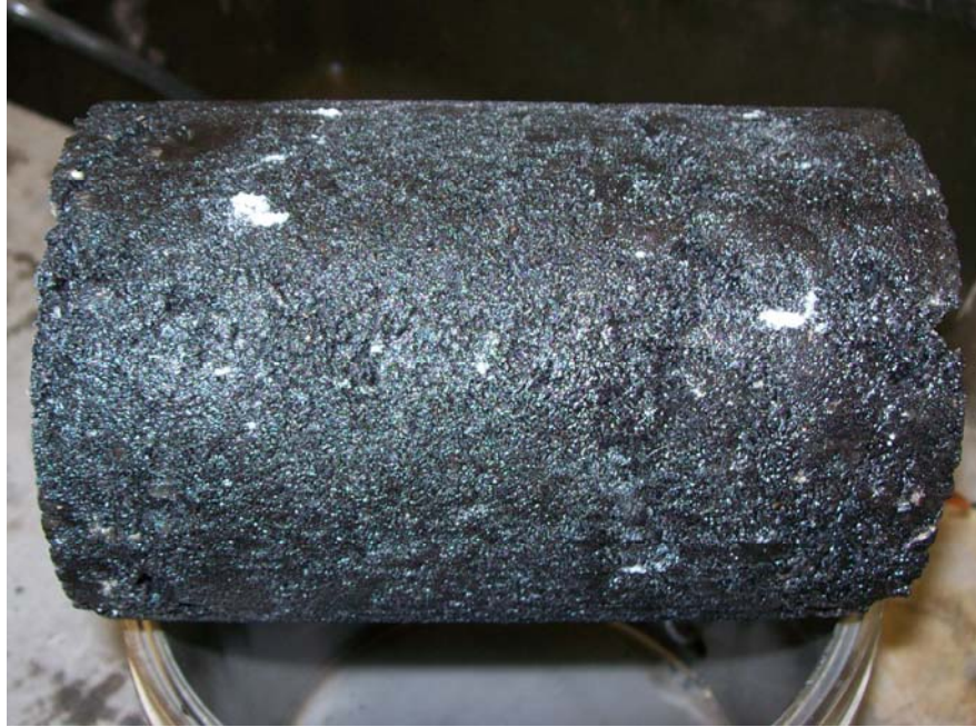
Figure 62. White Deposit on Exterior of Compacted HMA made with ED RCA Tested in Deicer Solution at 60°C
