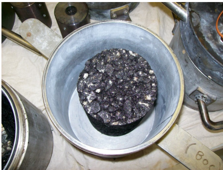
Figure 19. Superpave Gyratory Specimen in Dilatometer
