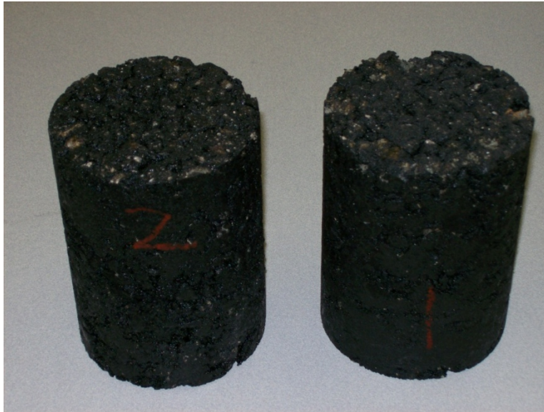
Figure 18. Superpave Gyratory 4 Inch Diameter Specimens
