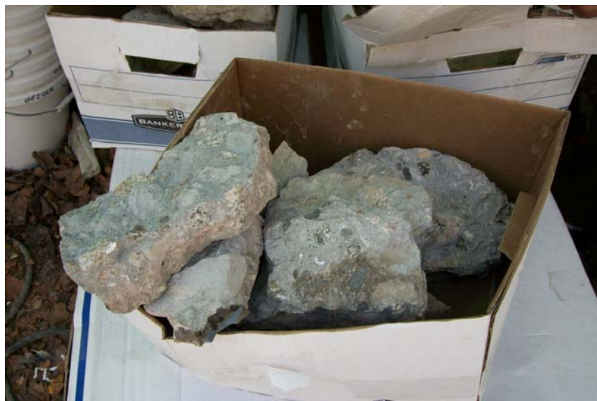
Figure 4. As-Received Edwards RCA
