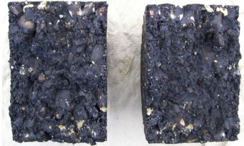
Figure 74. Fracture Cross-Section of Chert Specimen Conditioned in Water for 24 Hours
