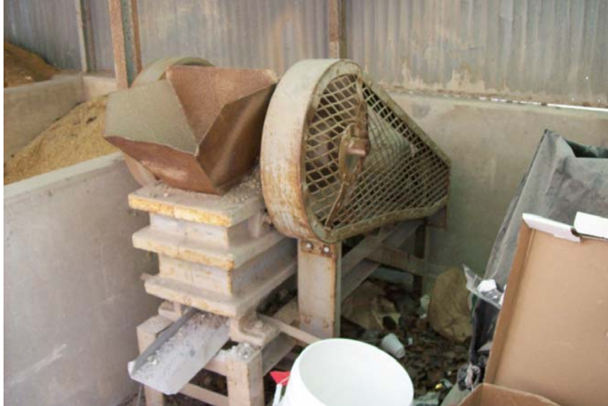
Figure 5. Jaw Crusher used to Crush RCAs
