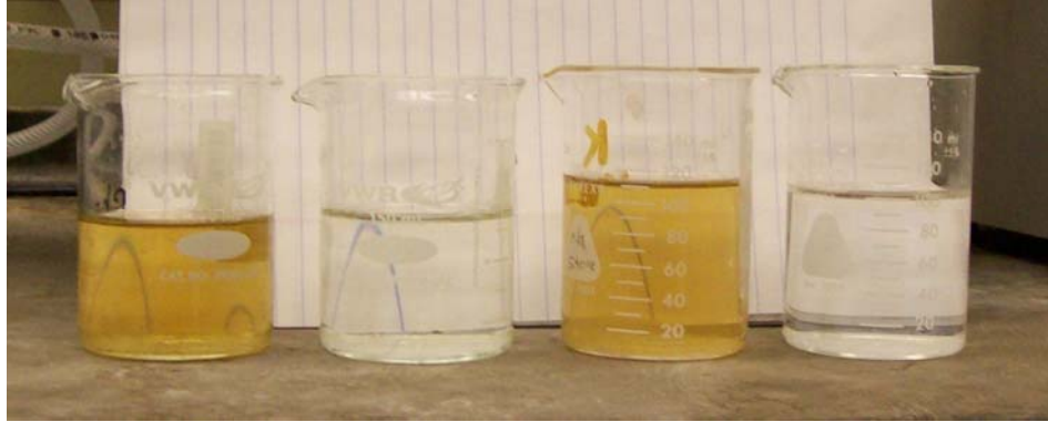
Figure 29. Water and Solution Samples from Compacted HMA made with Chert Tested in 0.5N NaOH+CH (L to R: 4.0% Binder in NaOH, 4.0% Binder in Water, 6.5% Binder in NaOH, 6.5% Binder in Water)
