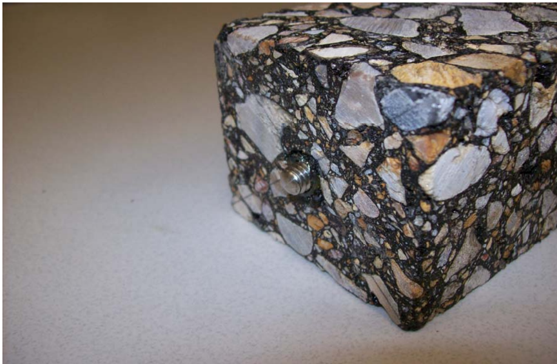
Figure 20. Measuring Stud Mounted in the End of Sample Beam
