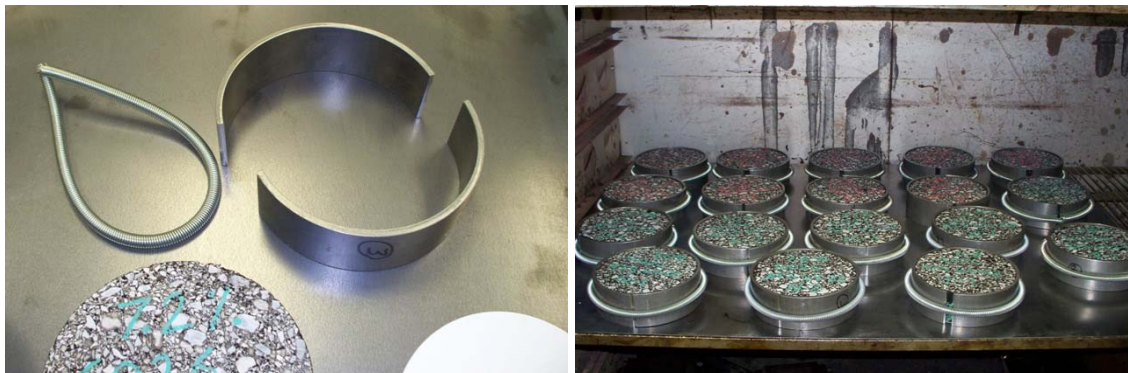
Figure 5-3. Long-term oven aging of laboratory compacted samples
