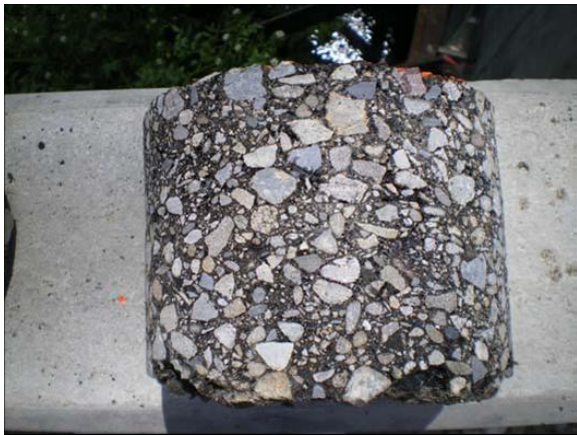
Figure B-51. Core #7 from Friedman Memorial Airport. Surface and binder course intact. Both the surface and binder course have fairly large aggregate.
