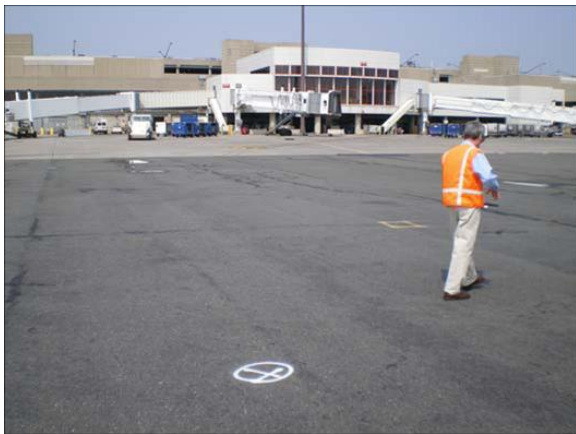
Figure B-15. Apron area in front of Boston Logan B Concourse near Gate B-28. Photograph taken in a high area of the pavement. Deicing fluid from the gate dicing operation likely flows onto this area but not as much as the location shown in Photograph 2. White dot indicates core location.
