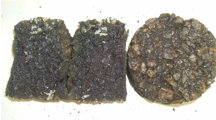
FIGURE 4.18 Lab Gravel Fuel Resistance Samples After Immersion.
