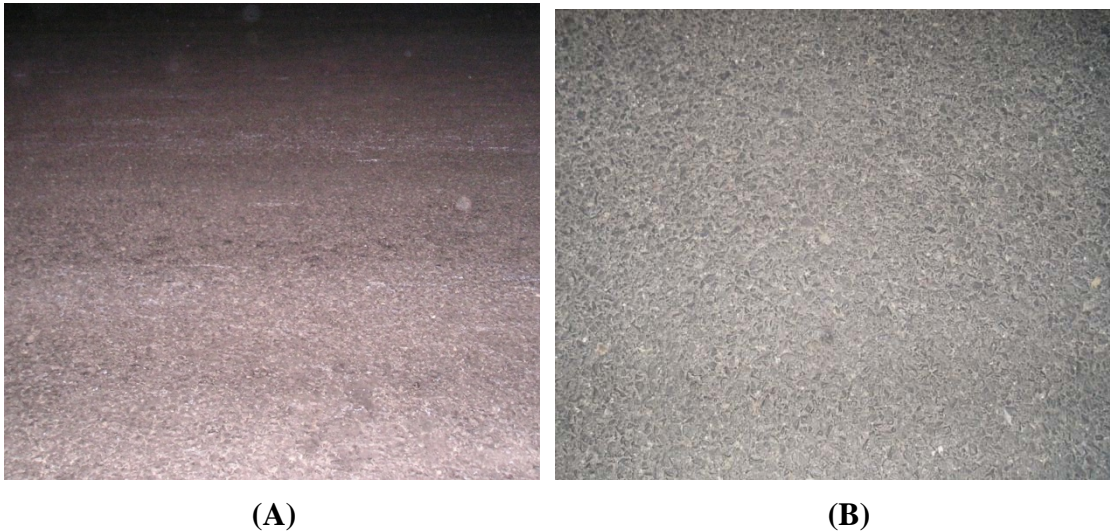
FIGURE 3.3 SMA Texture on East Runway (A) and West Runway (B).
