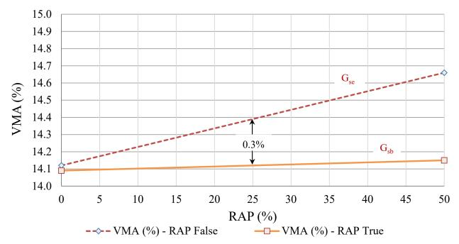
Figure 3. Comparison of reported VMA when using both G<sub>sb</sub> and G<sub>se</sub> for the same mixture.
