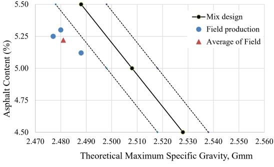
Figure 5. Relationship Between G<sub>mm</sub> and Asphalt Content.
