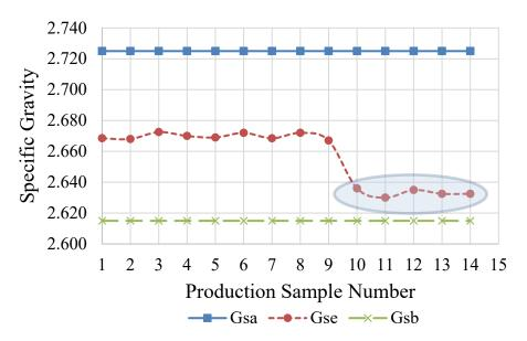
Figure 4. Aggregate Specific Gravities Control Chart.
