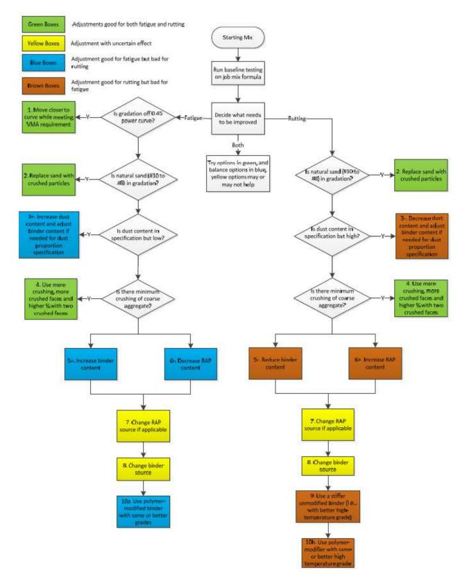
Figure 4. Chart. Revised flowchart proposed for improving the fatigue or rutting performance of an asphalt mixture (UCPRC-RR-2017-12).
